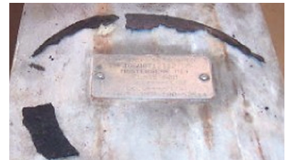
These pieces are all that remain after the Belleville springs dissolved in a competitor's super duplex valve.
