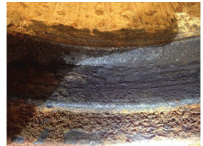
Material loss in the seat pocket was caused by galvanic corrosion, allowing leakage around the valve seats.
